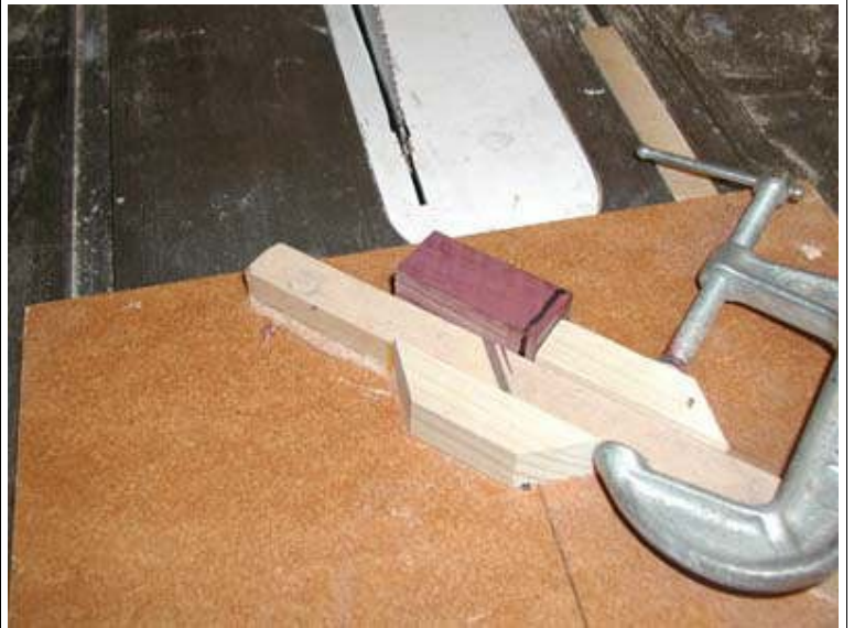
Set-up for 1st Cut - Note alignment "stripe"
