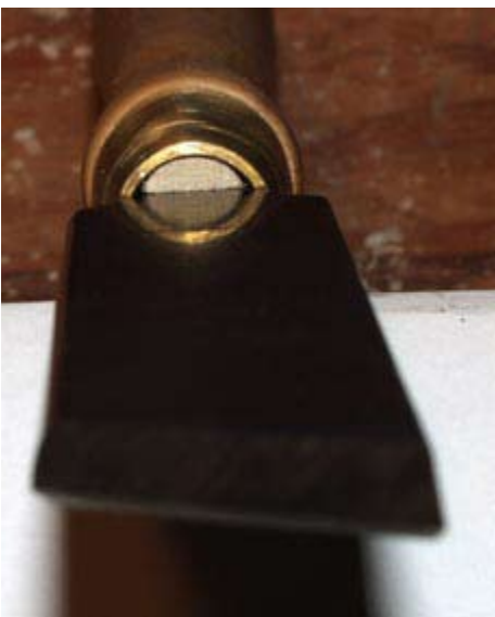
View of the finished handle for the skew showing the half-moon shims used to strengthen the handle at the ferrule. The epoxy hasn't been added so as not to obscure the view of the shims.
