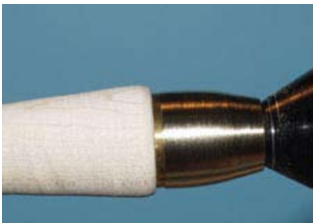
Fairing nut after filing the shoulders off and filing it round.
