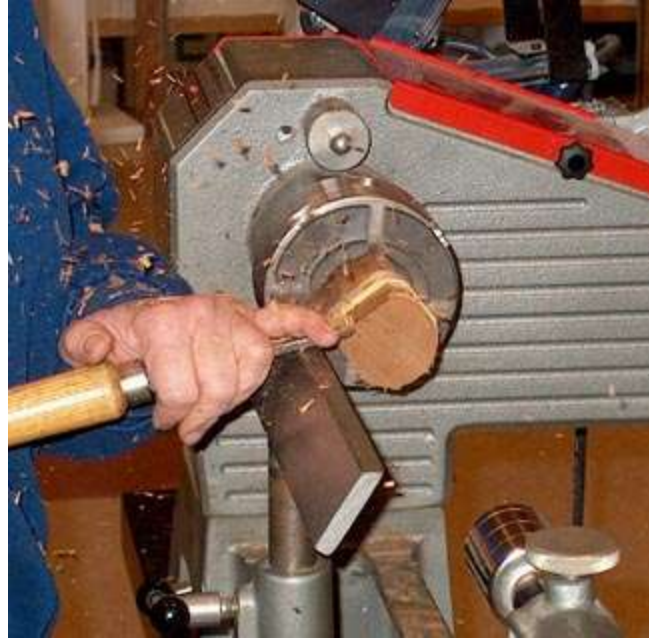
Roughing the blank to make it round
