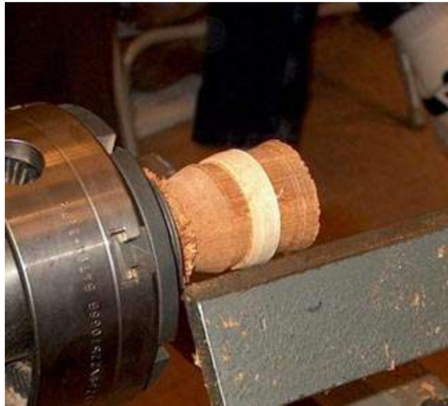
The wood on either side of the ring is tuned to a smaller diameter than the ring.
